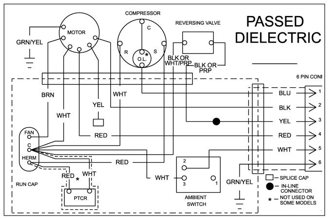
TYPICAL MECHANAL PENGUIN HEAT PUMP WIRING DIAGRAM
