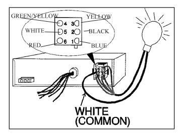
When the thermostat calls for that function and the Circuit is completed the light will illuminate.
