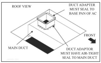
Restrictions at the connection to the air conditioner is the most common, but blockage in the main duct runs can also cause freeze-up. Blockages commonly occur in the areas where the duct changes direction. Other obstacles that can cause a change in the duct (air) path include rafters, vent pipes, wire bundles, etc.
