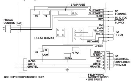
Wiring Diagram for 3107541.017 Cool, Furnace & Heat Strip 3107228.003
