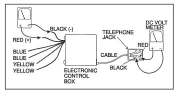
To check DC voltage at the thermostat , remove from mounting bracket. At the back side of the thermostat above the RJ-11-6C4P jack are four solder points where DC input can be checked.
