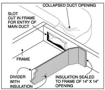
The final method of installation dumps the discharge air directly into the RV's main duct. The duct is routed through the 14-1/4'' x 14-1/4'' ( $\pm 1/8''$ ) opening. A duct adapter is used to connect the air conditioner to the main duct. If this connection is not made properly, cold air can migrate back into the return air path and make conditions right for freeze-up. Be sure the duct adapter is sealed to the main duct and air conditioner.
