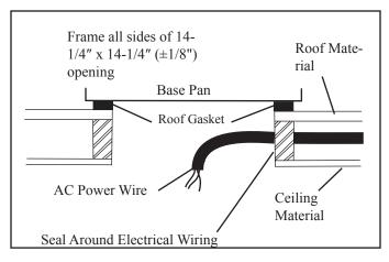
The most commonly found installation problem is the improper sealing of the  $14-1/4" \times 14-1/4" (\pm 1/8")$  opening in the roof cavity. The cooled discharge and warm return air are mixed in the roof cavity and produce conditions that are excellent for frost production.
