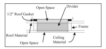
Another method of connecting the discharge air to the coach's main duct uses Duo-Therm's return air kits. One-half of the 14-1/4" x 14-1/4" ( $\pm 1/8$ ") opening is discharge plenum and one-half is return air plenum. If the duct openings are not clean, restriction of air can cause the coil to freeze. The opening of the duct should be as large as possible to make the air distribution better in the coach and reduce freeze-up.
