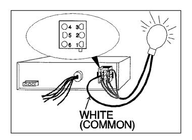
To verify circuits are being completed by the Single Zone LCD control board/box, you would first disconnect the 6-pin plug connector from the Single Zone Control Box. Using a 115 volt AC incandescent bulb, check from terminal 5 (white-common) to the other terminals to determine if a particular circuit is completed through the Single Zone Control Box. If the circuit is completed, the light will illuminate.
