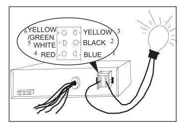
Note: DO NOT use a voltmeter to do these checks as it will give erroneous readings. If the circuit is completed (light bulb coming on) and a component is not operating, the problem is in the rooftop unit/wire harness.
