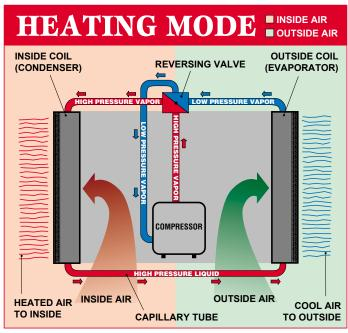
As the high pressure liquid leaves the inside coil (condenser) it passes through the small capillary tube or tubes, which act as the metering or flow control device in the sealed system.
