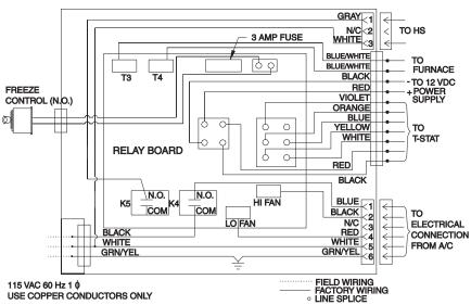
Wiring Diagram for 3107546.008 Cool, Furnace & Heat Pump
