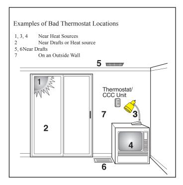
The proper location for the thermostat or remote sensor is 54" from the floor and on an inside wall. It should be located where it cannot be affected by heat from the sun, lamps, ovens, etc., or other sources of draft. Locations close to entry doors and windows should be avoided. The discharge from registers blowing directly on the thermostat or remote sensor can cause the systems to short-cycle and should be avoided.
