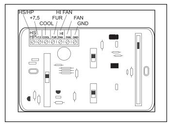
If any one of the volt readings is missing, check T-stat cable to control board. If the voltages shown above are present, use a jumper wire to test unit operation as follows: This test will bypass the function of the thermostat. The thermostat provides a ground to close a relay.
