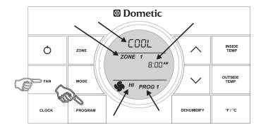
When program 1 or 2 is operating, the "PROG 1 or 2" icon will be displayed in the LCD. The zone will continue to operate in the programmed setting until the program is manually cancelled. To cancel the program operation, press and hold the PROGRAM button for 3 seconds. The zone will be restored to normal operation.
