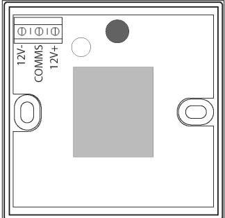
NOTE: There is no DC fuse on the main control board, if the DC control amperage exceeds 1.5 to 3 amps the DC voltage will be shut down. To reset the PTC disconnect the DC power source positive wire for 30 seconds and reconnect.
