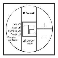
The Single Zone LCD thermostat is equipped with both a liquid crystal display (LCD) that identifies the temperature set-point, fan speed (Auto, Low, High), and F/C and green LEDs that indicate the mode of operation (Off, Fan, Cool, Furnace, Heat Pump or Heat Strip\*). The
