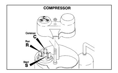
Use an ohmmeter to check for continuity through the overload device. If no continuity is found and the compressor is hot, allow 15 to 20 minutes for the compressor to cool. If a repeat of the test shows the overload to be open, it is defective and requires replacement. Note on some 15,000 BTU units the overload may be an internal component and non replaceable.
