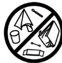
**CAUTION!** Flush only water, bodily wastes and rapid-dissolving tissue paper. Do not flush wet wipes, sanitary napkins, condoms, diapers, razor blades paper cups, cotton swabs food, hair or liquids such as oils or solvents. Clogging or damage to the toilet system may occur.
