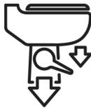
Press foot pedal sharply down until contents clear bowl. (A popping noise is normal when the vacuum seal is broken.) Hold foot pedal for three seconds. After flush, let foot pedal snap back into position. If foot pedal is accidentally released before waste clears bowl, do not flush again until vacuum pump stops running. A small amount of water remains in bowl after flushing.
