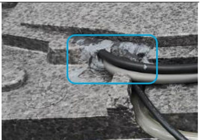
2. Organize 1 pcs of sealing compound (3) and seal the passage of the condensate hose in the housing with.
