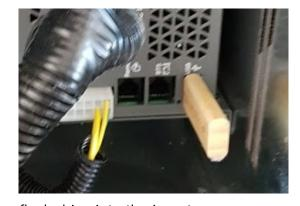
Plug the flash drive into the inverter
