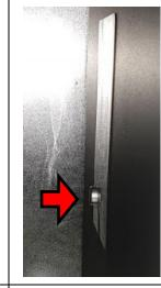
Ensure the inverter is turned on by depressing the button and making sure it is ON on the Dometic Touchscreen.
