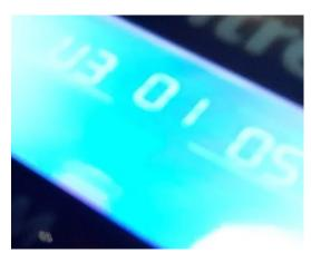
Verify the update took place by using a mirror to view the inverter display. And press the middle button on the display until you see a "U3 01 05" displayed.
