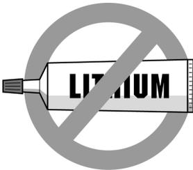
**LITHIUM-BASED GREASE** has led to cracks in adapters due to chemical reaction with certain PVC formulas.
