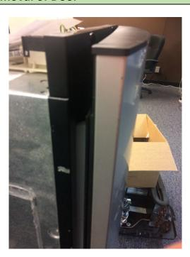
2. Locate the 3 screws on the top of the fridge that are connecting the top door hinge to the fridge
