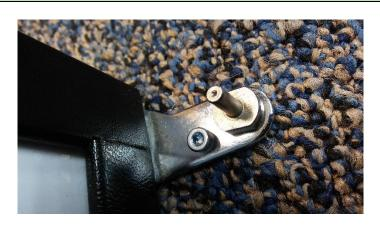
2. Locate the trim screw on the bottom right of the door ( Bottom Left of the door for a left sided hinge, Always opposite of handle side)
