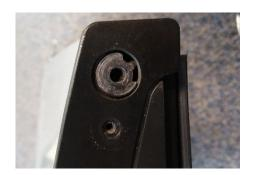
4. Place the new door stop piece on the door and screw down using the new 4x20 screw that was included in the kit
