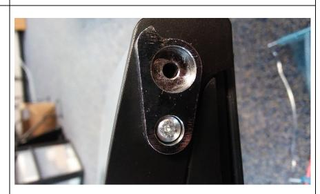
5. Once door stop piece is attached to the door, place the bottom of the door onto the new pin on the bottom hinge
