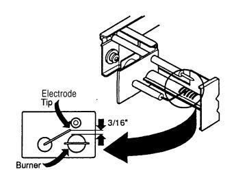
NOTE: If igniter (see Section 4.12) and high voltage cable (see Section 4.14) are good and there is no spark at the tip of the electrode, REPLACE THE ELECTRODE.
