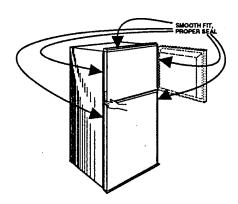
To correct door alignment, loosen the hinge screws slightly and re-orient the door in the proper position. Hold the door in its new position and carefully re-tighten the hinge screws.
