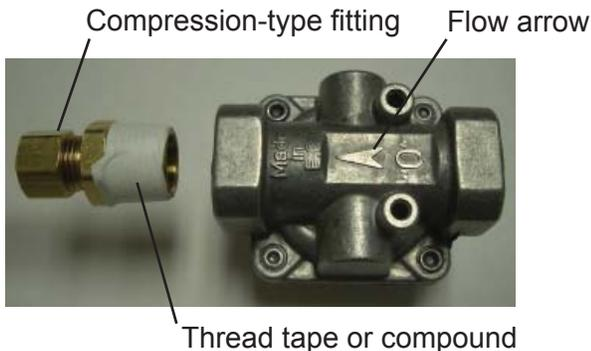
2. Thread the 3/8" NPT end of the flare-type fitting into the inlet end of the regulator, applying thread tape or sealing compound as noted above. Tighten using appropriate wrenches. Remember that the top caps on the regulator must be accessible once the installation is complete, so align any elbow fittings involved with that in mind.
