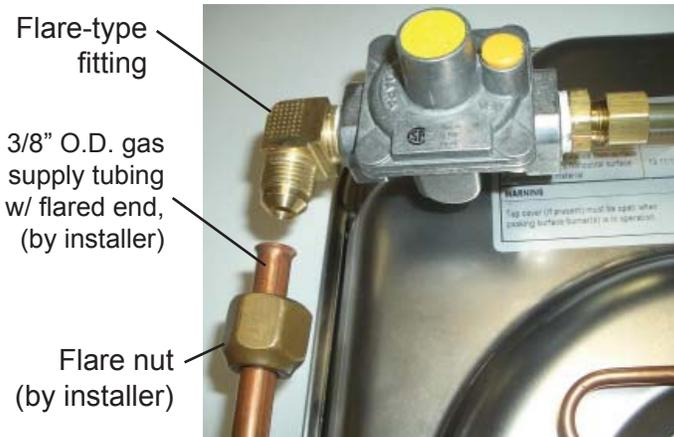
5. **IMPORTANT:** The gas supply tube, whether flexible or rigid, must be securely supported by a clamp (supplied by the installer) at a point no further than 6 inches from the connection to the pressure regulator. The supporting clamp may not be attached to the cooking appliance itself. This is required in order to maintain compliance with safety regulations.
