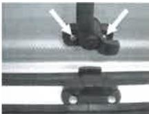
Loosen rotary clamp at the fixing screws and install new part in reverse order.
