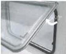
With fixing in a new acrylic pane, it must be ensured that the windowpane hinge is positioned properly in the frame hinge. With fixing the windowpane, the fitting angle must be  $>90^\circ$ , so that the windowpane hinge can be inserted into the frame hinge. Before closing, ensure freedom of movement in order to avoid possible damage in the hinge area. Then close window and fasten opener to the frame.
