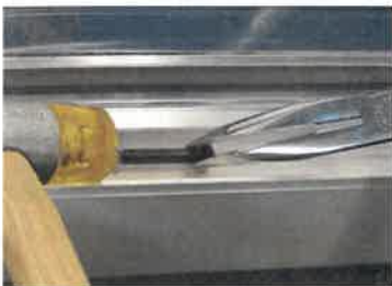
5.) Catch the hinge- pin with the pliers and pull; if necessary hit the pliers with a rubber mallet.
