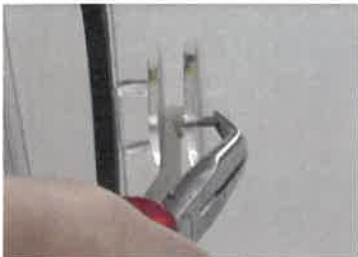
3.) Remove the bolt with a pointed plier.
