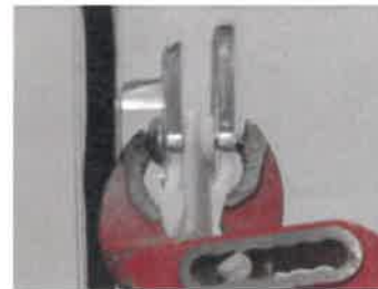
11.) Press the cap with a tong to the bolt.
