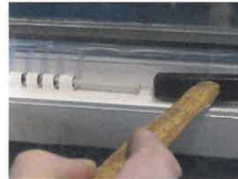
9.) Beat the hinge-pin into with a hammer.
