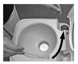
3. Place guide wire through small hole in bowl and route through upper tank to bellows pump hole.
