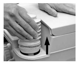
Remove pump body and hose assembly from tank by twisting to loosen sealant and pulling out pump. If pump cannot be loosened and removed easily, cut through sealant or pump at base (be careful not to cut tank).
