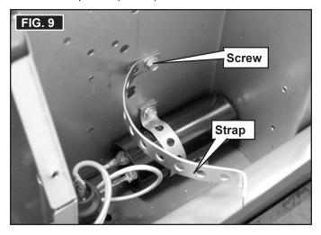
4. Place both capacitors in position and secure with strap and screw. See (FIG. 10).
