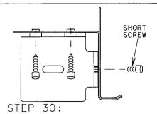
MOUNT AN INVERTED ATTATCHMENT ON THE OTHER SIDE OF THE REFRIGE-RATOR.
