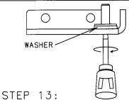
USE A SCREWDRIVER TO LOOSEN THE PIN. REMOVE THE PIN AND THE WASHER. THROW AWAY THE HINGE.
