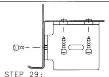
REMOVE THE 3 SCREWS FASTENING THE ATTATCHMENT FOR TOPDECOR. SAVE THE SCREWS AND THROW AWAY THE ATTATCHMENT.
