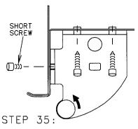
MOUNT THE TAP OF THE UPPER DOOR HINGE IN THE BUSHING OF THE DOOR (UPPER DOOR). TURN IT TO-WARDS THE FRONT FRAME AND FASTEN THE SCREWS.
