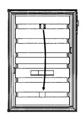
BEFORE DRILLING NEW HOLES AT THE LOWER PART OF THE DOOR USE THE CENTERATTACHMENT AS A MASTER TO MARK UP THE POSITION OF THE NEW HOLES USE A DRILL WITH DIAMETER 4 MM.
