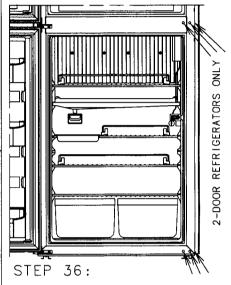
MOUNT PLUGS IN THE HOLES NOT OCCUPIED BY THE HINGE (HINGES).
