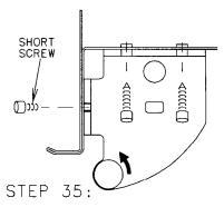
MOUNT THE TAP OF THE UPPER DOOR HINGE IN THE BUSHING OF THE DOOR (UPPER DOOR). TURN IT TO-WARDS THE FRONT FRAME AND FASTEN THE SCREWS.
