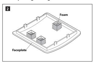
➤ Remove any distorted or deformed foam.
