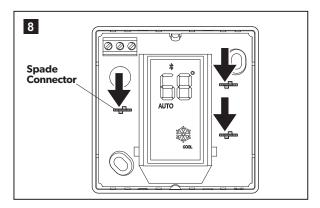
➤ If the unit does not respond, remove the touch panel faceplate and operate the spade connectors directly by finger to control the unit.
