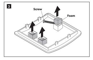
➤ Use a pointed, but not sharp, object to carefully pry out the distorted foam from its cavity without damaging the foam or the cavity.
