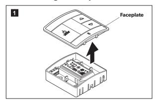
➤ Power off the unit and remove the touch panel faceplate.
