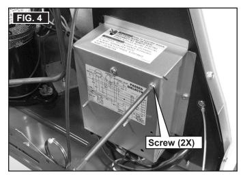
6. Remove screw to loosen capacitor retaining strap. Save for reinstallation later. See (FIG. 5).
