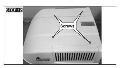
Once all locations have been properly sealed, re-attach the shroud by replacing and tightening the four screws removed in STEP 6.
