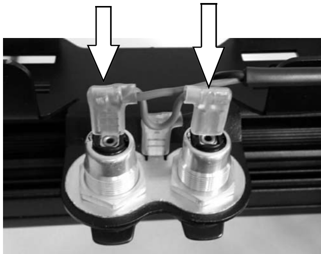
Red Wire to "tab" in center of Hella Plug
