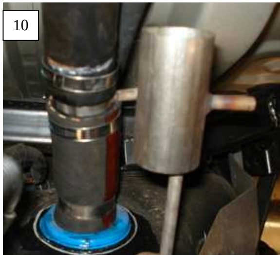
16. Fit 100mm long filler hose supplied to the main tank. Insert T-piece and join to main hose. (Pic 10)
