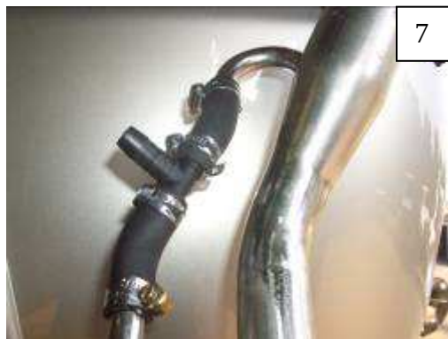
13. Insert plastic T-piece supplied using clamps and short pieces of hose as shown. (Pic 7)
