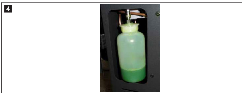
Fig. 4: Waste oil collecting tank of the A/C service station
