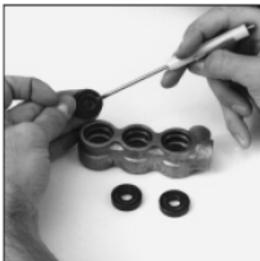
Installation of Lo-Pressure Seals
