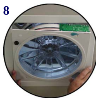
Install New Control Panel
