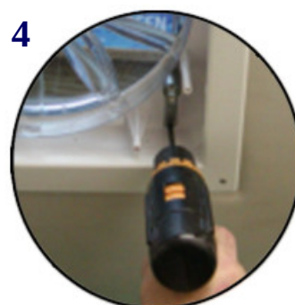
Unscrew the Lift-Arm ASM
