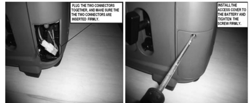
STEP3: PLUG THE TWO CONNECTORS TOGETHER
